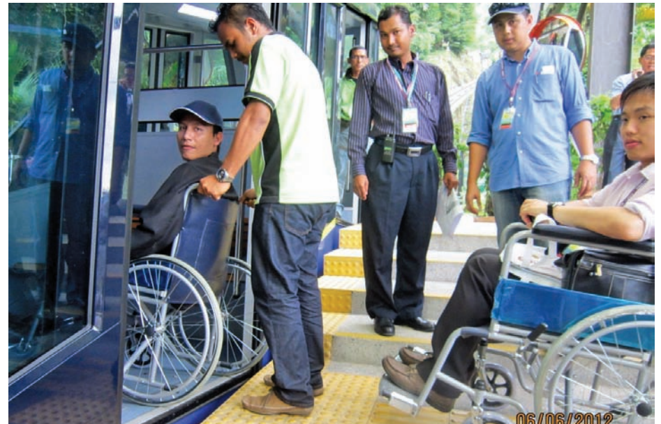
The Penang Hill furnicular train is accessible to wheelchair users and has tactile blocks for the visually impaired (yellow tiles on the floor).
