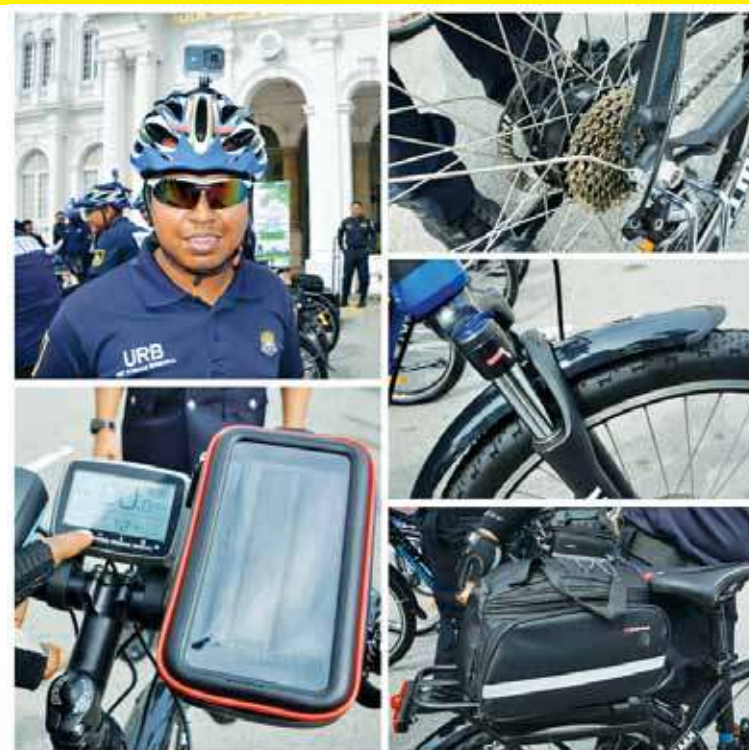
(Clockwise from top left) An officer wearing the helmet which has a GPS trip recorder with an action camera attached on its top, the speed gear transmission, advanced suspension system, battery pack and speed controller.
